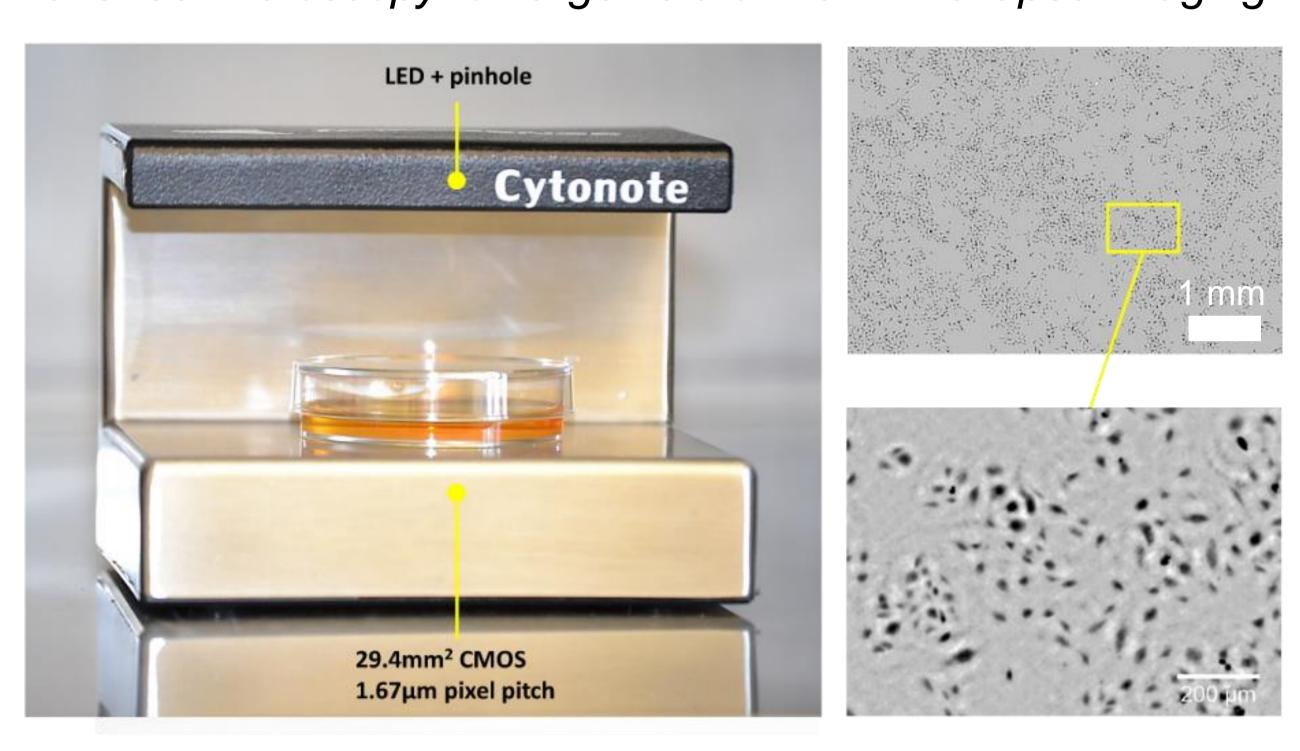
Experimental setup of the lensfree video microscope (2014 IPRASENSE Cytonote). (Left) A CMOS image sensor is used for image acquisition and an LED and a 150 µm pinhole for illumination (5 cm above the image sensor). (Right) Acquisition and phase reconstruction of a culture of primary human umbilical vein endothelial cells (HUVEC) (scale bar 1000 µm). The field of view is 29.4 mm2 and contains about 4000 cells.
